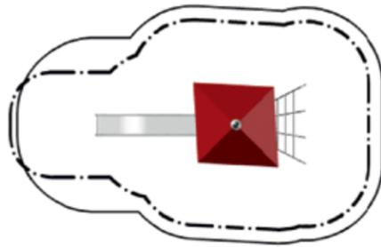
Shack1 with a landing height of approximately 5' is the smaller one of the two play huts. In this variation, the "witch's house" distinguishes itself through its high transparency. The two different entrances can be climbed into using the slanted net ascent, as well as a climbing rope with rubber cylinders which function as a climbing support. A special feature of Shack1 are the posts that are slanted outwards.
