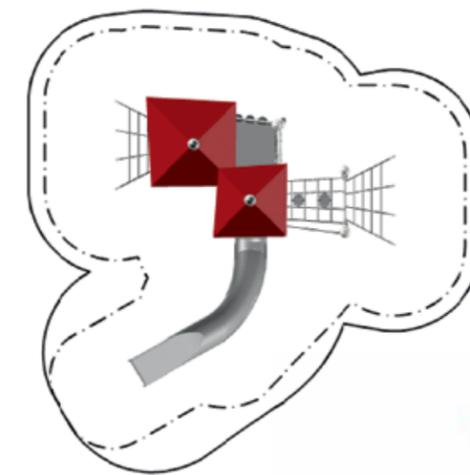
The Woodville Combi.02 combines 2 huts of different heights, which share a common support post. The larger of the two huts is equipped with a connecting mesh net, which is combined with an entry net, and thus offers an exciting challenge. The two huts are connected by a balcony which can be climbed via a rope ladder or using the rocking-plate ascent.
