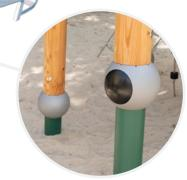
The system balls made from aluminium are a tried and tested connection element of Berliner. The steel posts are thus elegantly connected to the wooden posts. The construction prevents the direct contact of the wood with the ground and thereby protects it from rot due to lasting moisture. An extra post shoe is therefore not needed.
