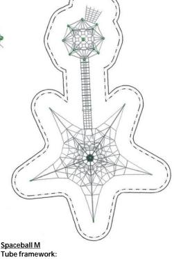
Frameworx-steel tubes, Ø 60.3 mm (2 3/8"); anti-corrosion treatment and color finish: sandblasting and solvent-free zinc-/ epoxy-/ polyester-process
